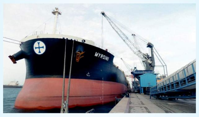
Coal being discharged from the vessel 'M.V. Myrsini' using Harbour Mobile
