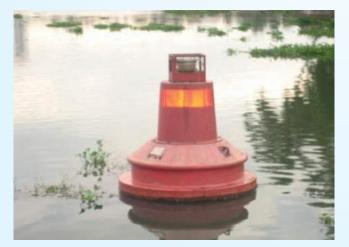
Solar Powered FRP Buoy installed in NW-3
